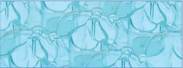
Figure 2: ThinCert™Plate: Notches (arrows) secure the position of the ThinCert™ cell culture inserts during cell culture.
